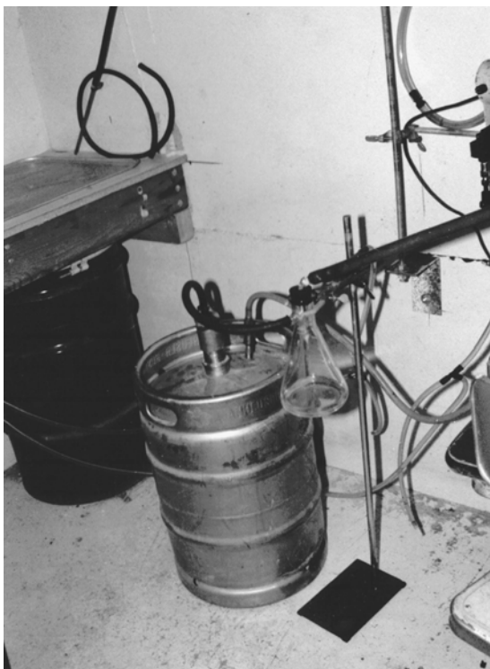
Figure 9.10 Homemade vacuum distillation apparatus.
