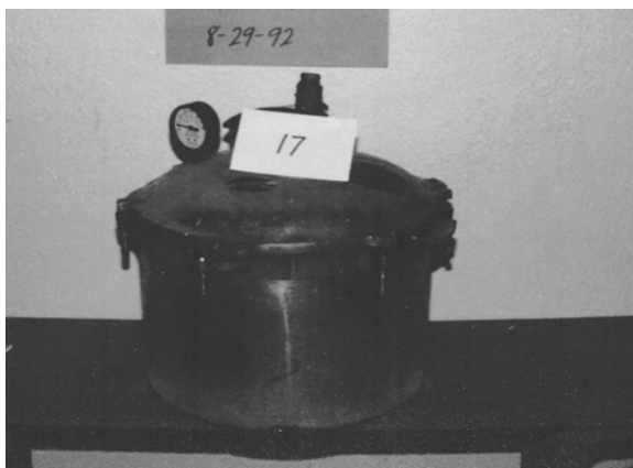
Figure 9.5 Pressure cooker reaction vessel.
