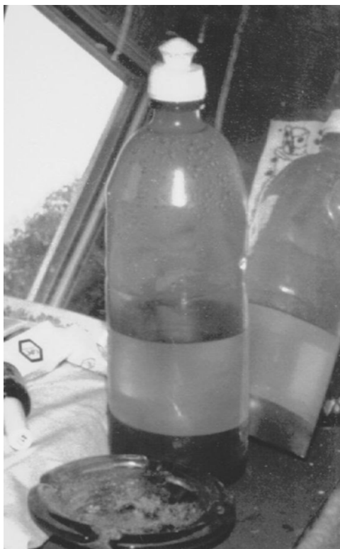
Figure 9.12 Plastic soda bottle used as a separatory funnel.
